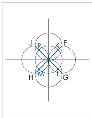
5. The straight lines both divide the circle into eight equal parts and locate eight equally spaced points—**B, C, D, E, K, L, M, P**—on the circumference of the original circle. This is the result of the five circles having the same radius. These points can be used to form octagons, eight-pointed stars, and four-pointed stars, as shown in Activity 5.
