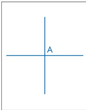
2. Place the compass point at point **A** and draw a circle. Leave room to draw equal sized circles on each side, at the bottom, and at the top. Mark the points that cross the lines **B, C, D, and E**.
