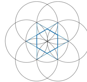
3. Connect opposite corners of the hexagon within the star. Extend the lines to the edge of the central circle to divide the star into twelve equilateral triangles. Erase the lines inside the central circle, leaving the circle and line end points visible.
